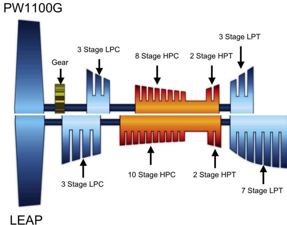
Figure 21: Engine Stage Comparison, PW1000G vs. CFM LEAP<sup>32</sup>
