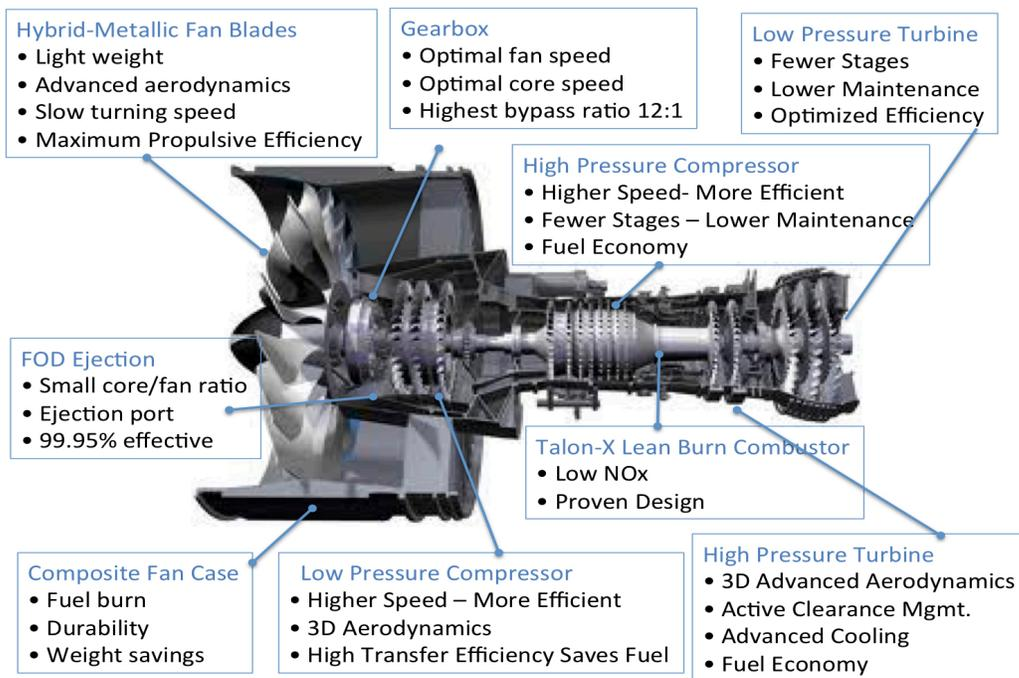
Figure 8: Diagram of Key Features on the PW1000G Engine
