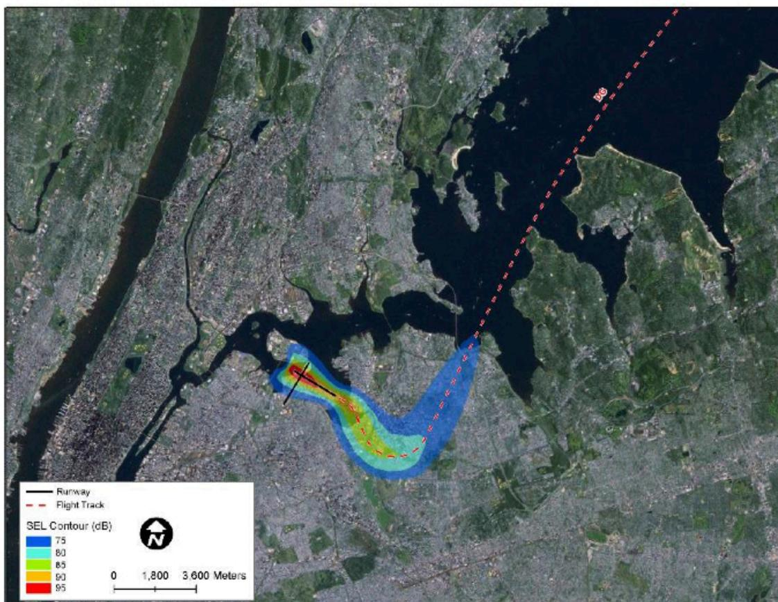
**Figure 17: Noise Footprint for PW1000G at LaGuardia Airport<sup>26</sup>**
