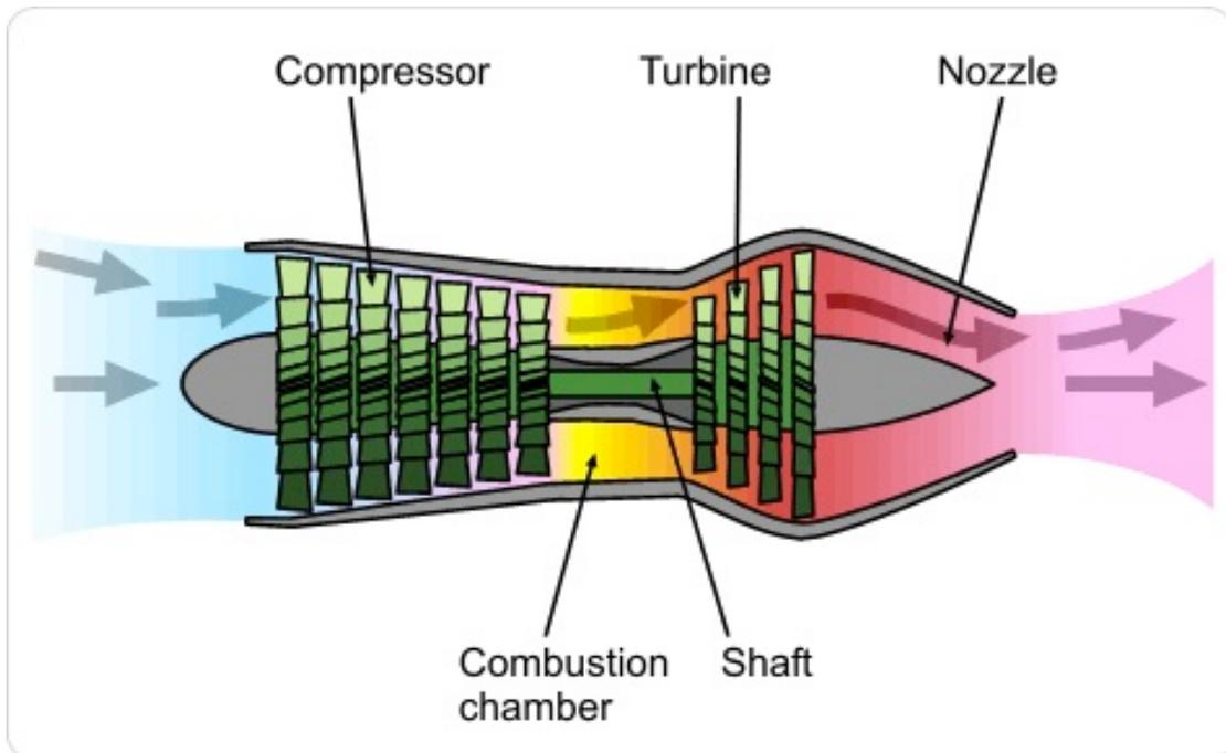
*Figure 4: The Configuration of a Turbojet Engine*
