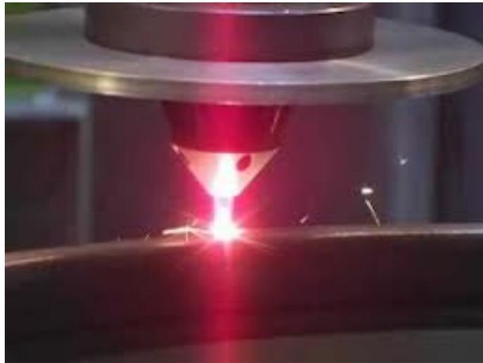
***Figure 9: Example of an Additive Manufacturing Process, or 3D Printing of Metal Parts<sup>11</sup>***
