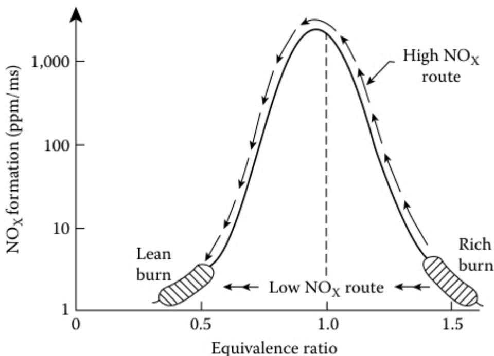
**Figure 15: Graph to illustrate the Principle of Rich-Burn, Quick-Quench, Lean-Burn (RQL) Combustion.<sup>23</sup>**
