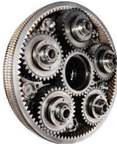
*Figure 7: Photo of PW1000G Gearbox<sup>8</sup>*
