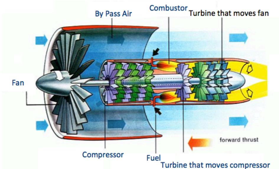
**Figure 6: Illustration of a High Bypass Turbofan**
