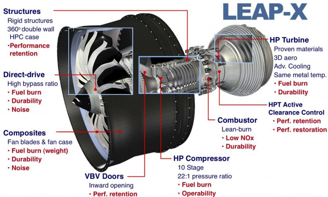
Figure 18: Key Features of LEAP engine<sup>27</sup>
