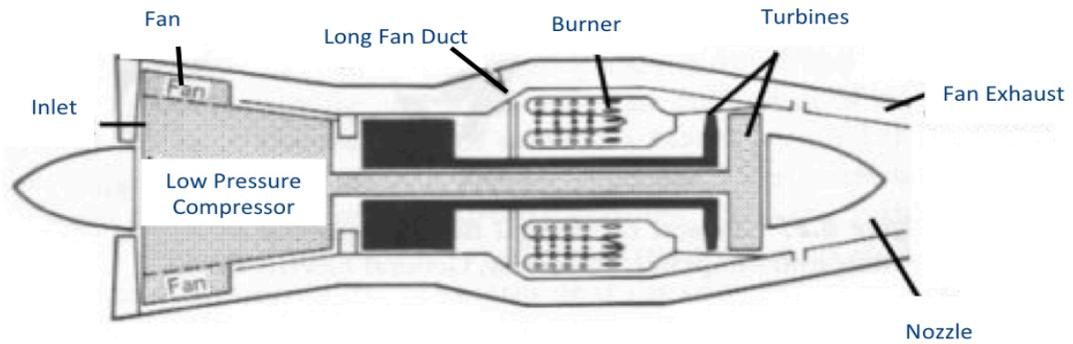
**Figure 5: Diagram of Low Bypass Turbofan**
