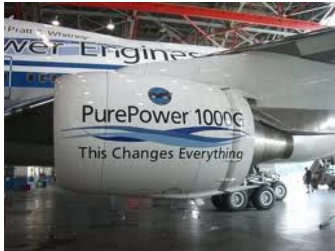
*Figure 1: Pratt & Whitney PW1000G Engine Prototype on Test Aircraft<sup>1</sup>*
