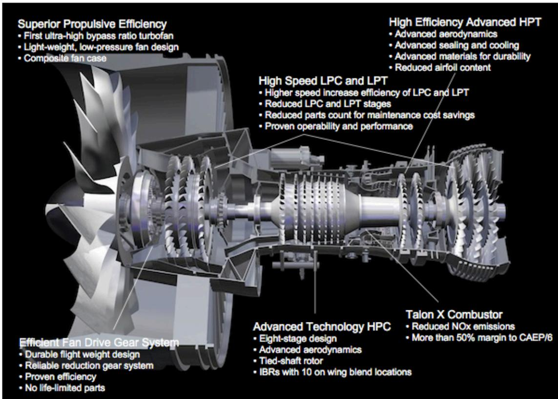
**Figure 19: Key Features of the PW1000G Engine<sup>28</sup>**
