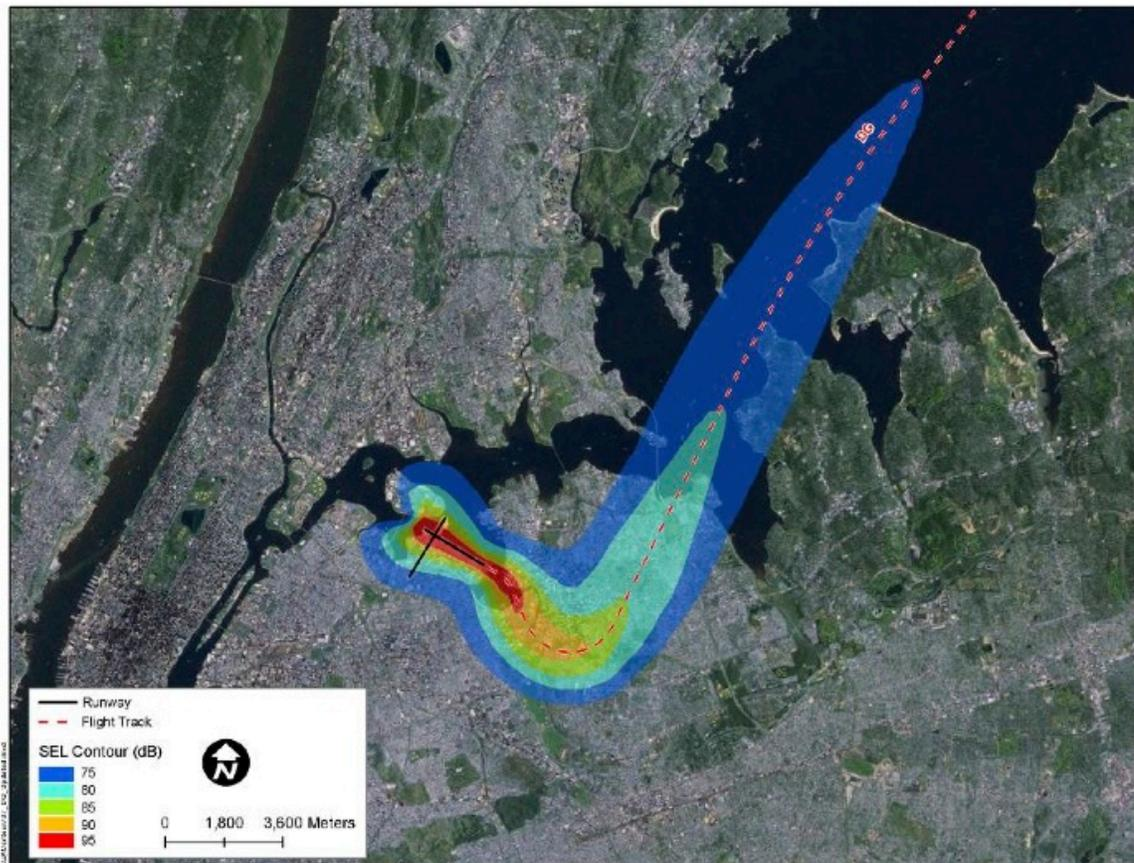
Figure 16: Noise Footprint for Today's Narrow-Body Engines at LaGuardia Airport<sup>25</sup>
