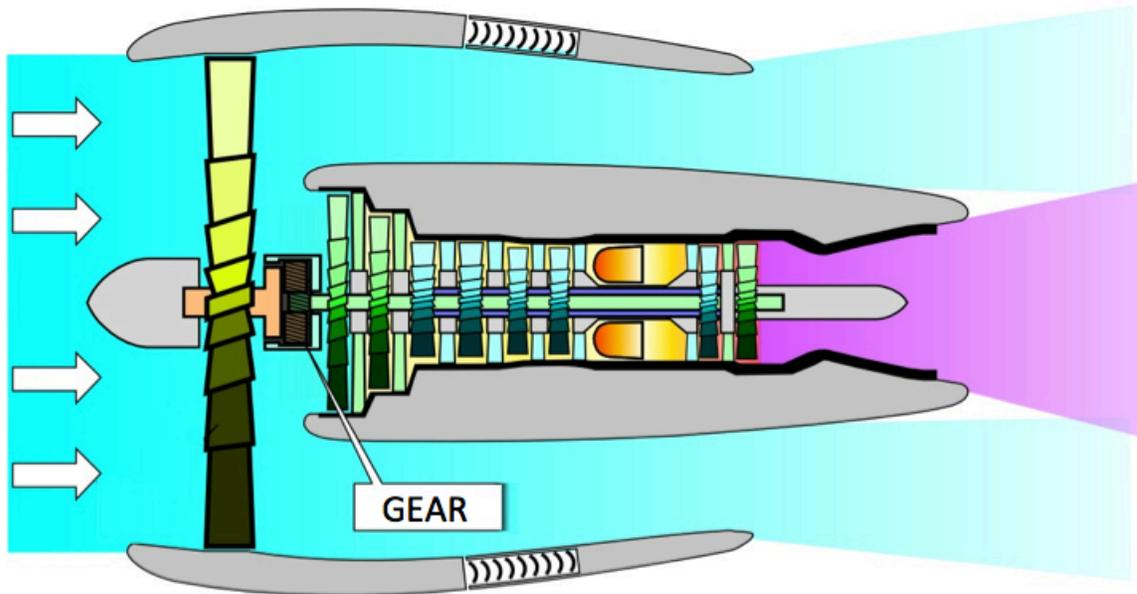
*Figure 2: Configuration of Geared Turbofan Engine and Position of Gear between Fan and Engine Core.<sup>4</sup>*
