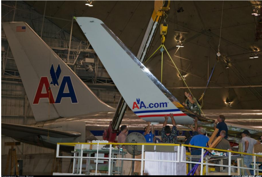
Photo Source: American Airlines. The after-market blended winglet reduces fuel consumption on the 767 by about 3.5%-4%.
