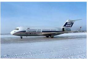
The TU-334 was meant to replace the TU-134. While the TU-334 was designed to be based on the latest thinking in terms of aerodynamics, structures, avionics, time may have passed it by. The Tu-334 has a high degree of commonality with the layout of equipment and aircraft systems with larger Tu-204/Tu-214. Indeed the flight decks are the same.
