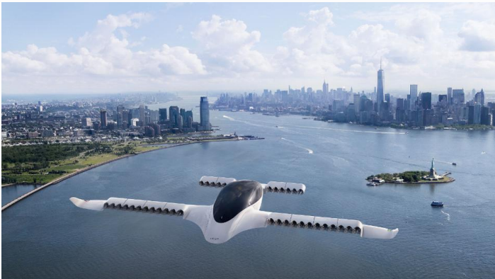
Lilium says its piloted electric aircraft will be able to carry four passengers and their luggage 186 miles at 186 mph. COURTESY OF LILIUM AVIATION
