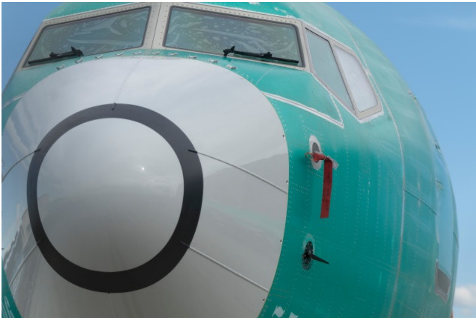
One of two sensors that measures the angle of attack is pictured at bottom on a Boeing 737 MAX 8 airplane outside the company's factory on March 22, 2019 in Renton, Washington (Stephen Brashear/Getty Images)
