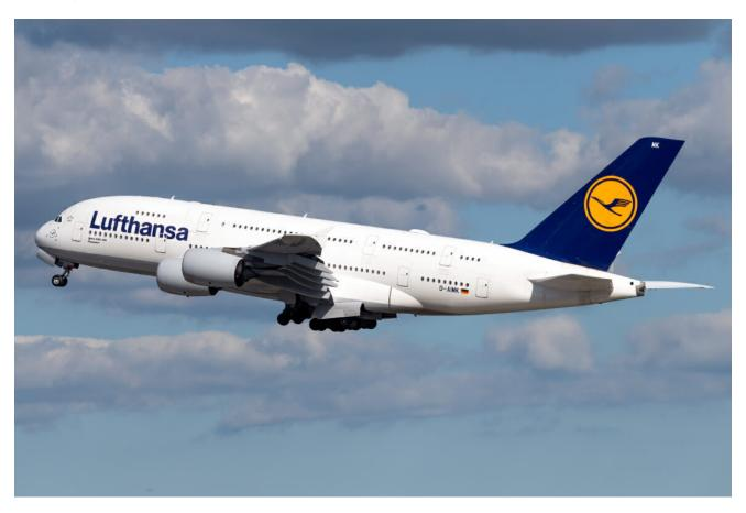
Controllers must leave sufficient space behind A380s to allow following aircraft to avoid its strong wake. Photo: Vincenzo Pace | Simple Flying.
