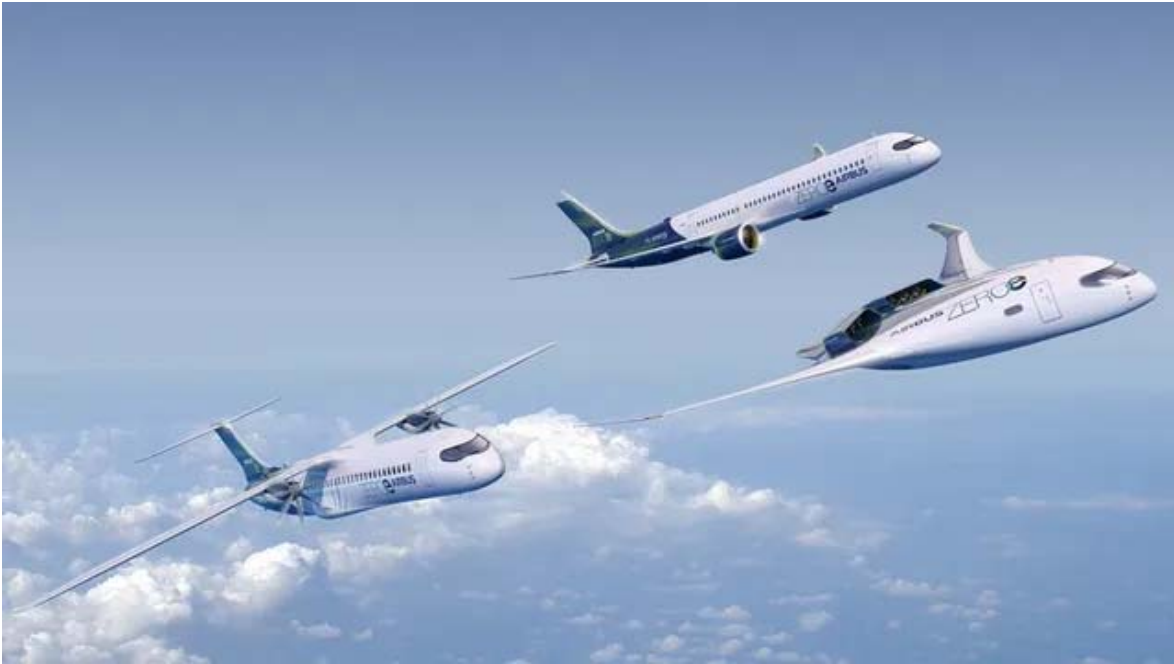
The three commercial aircraft designs of Airbus, using hydrogen as a mode of propulsion. (Airbus SAS 2023)
