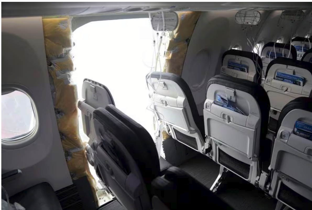
A panel used to plug an area reserved for an exit door on the Boeing 737 Max 9 jetliner blew out shortly after the flight took off from Portland, Oregon. AP
