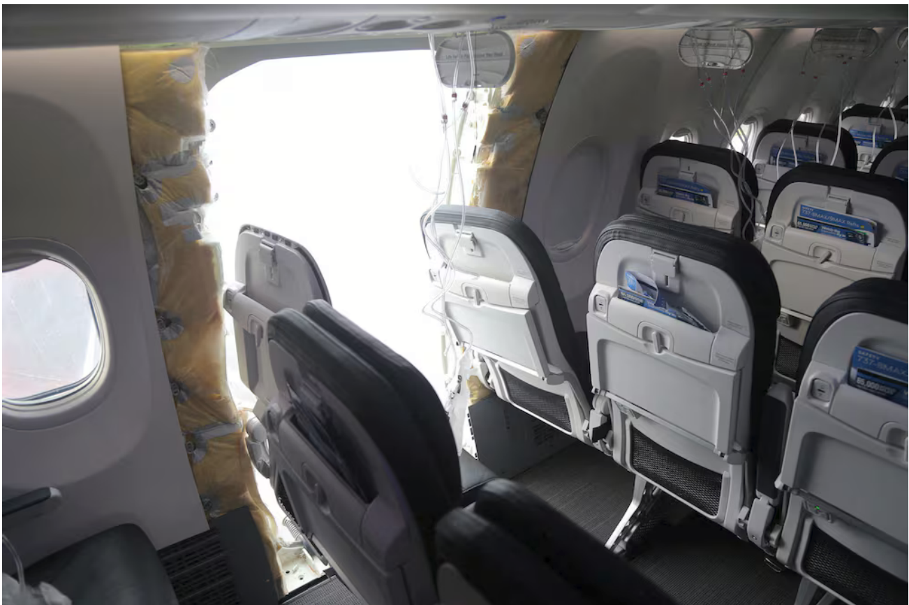
The fuselage plug area of Alaska Airlines Flight 1282 Boeing 737-9 MAX, which was forced to make an emergency landing with a gap in the fuselage. Reuters
