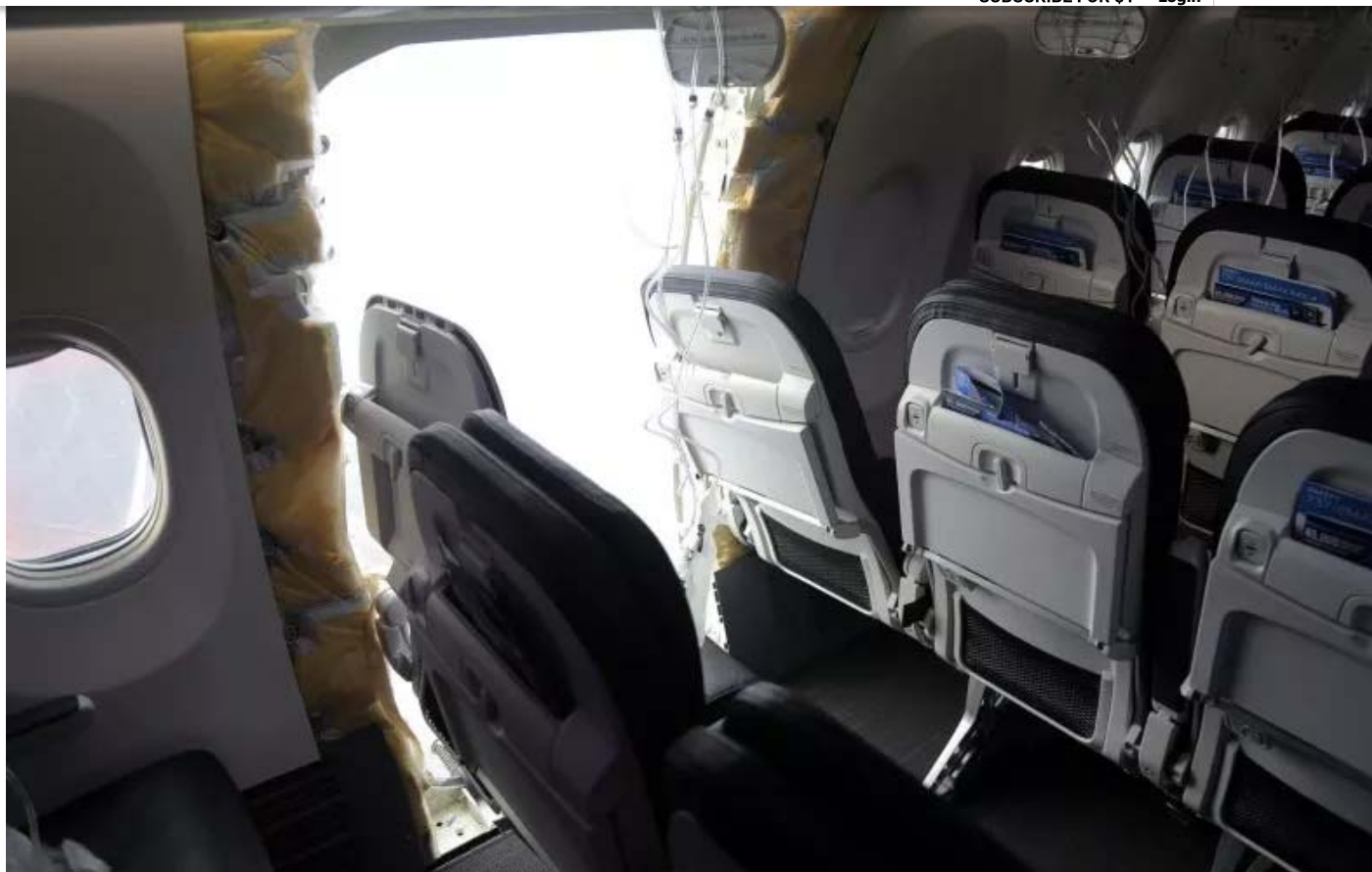
In this National Transportation Safety Board (NTSB) handout, an opening is seen in the fuselage of Alaska Airlines Flight 1282 Boeing 737-9 MAX on January 7, 2024 in Portland, Oregon. A door-sized section near... More NTSB VIA GETTY
