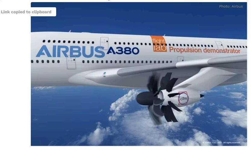
It seems the next generation of narrowbody engines will look like turboprops. CFM International is working on the RISE Program that will serve as the foundation for the next CFM engine generation. It is operational in the late 2030s and plans to improve fuel ef
